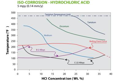
Tantalum and niobium are highly corrosion-resistant metals that are virtually inert to acid attack. These reactive metals outperform other materials, drastically reduce downtime, and add years of service life to process-exposed equipment.
