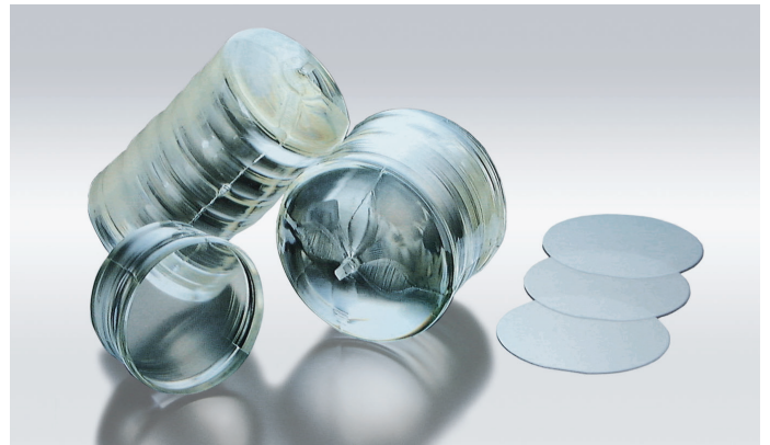
Sapphire crystal boule produced from crystal growing process.
