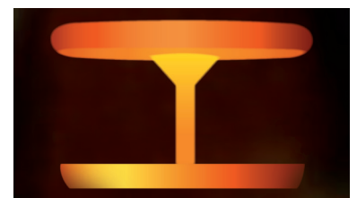
Red hot isothermal forging die
