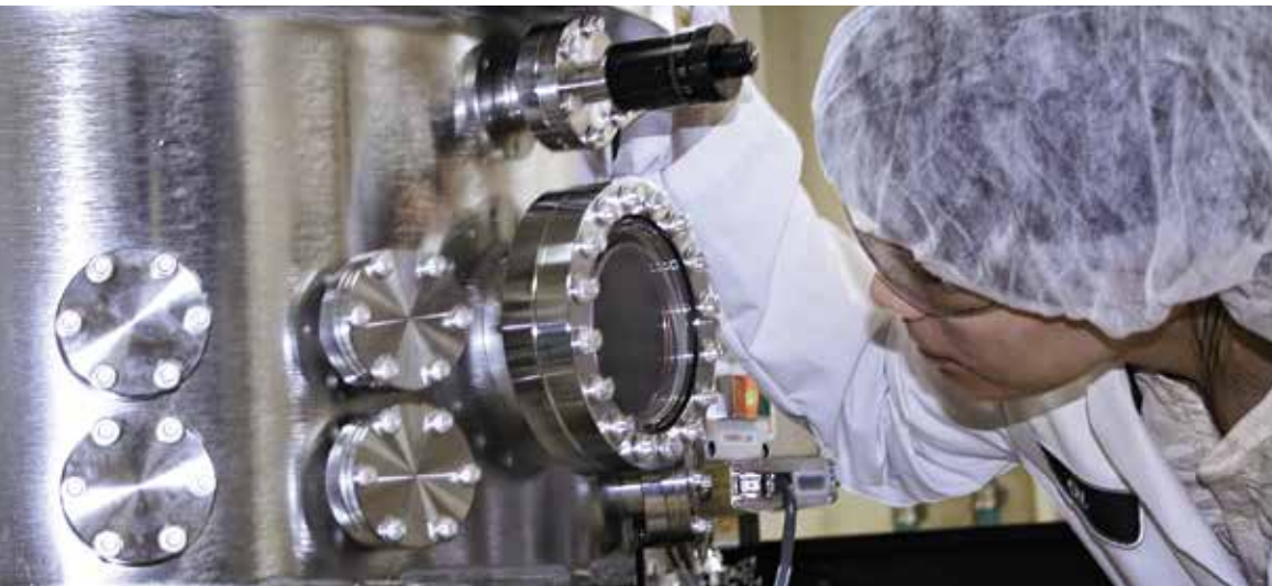
H.C. Starck Solutions' thin film laboratory is capable of sputtering experimental targets under a wide variety of conditions.
